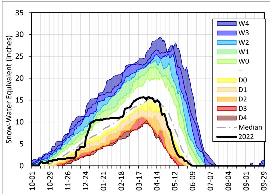
Figure 12: Snow water equivalent precipitation chart for the current water year, superimposed on percentile ranges matching the drought and wetness classifications [9].
