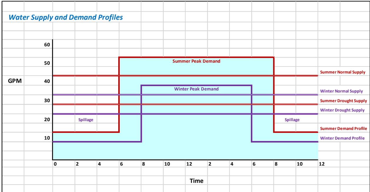
Figure 4: Estimate of water supply and demand profiles under both normal and drought conditions.
