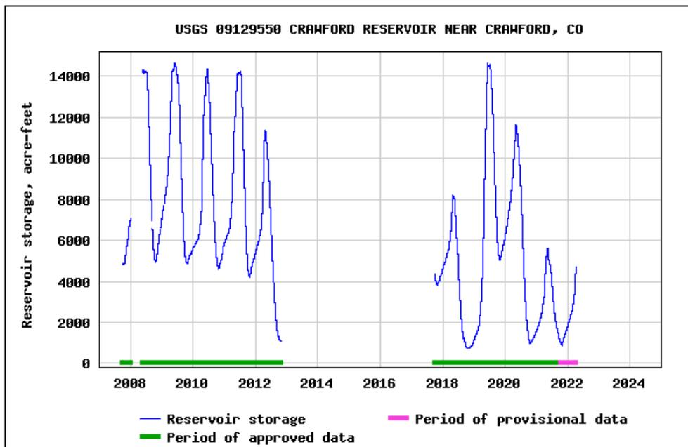
Figure 11: Storage volume measurements in Crawford Reservoir [14].
