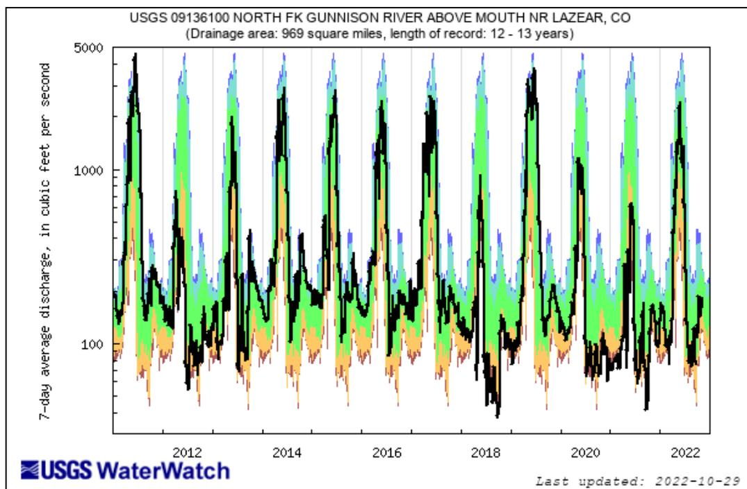
Figure 9: Streamflow seven-day averages measurements at gauge #09136100 "North Fork Gunnison River. It is on an adjacent tributary to Smith Fork where the DDWC Spring Box is located [14].
